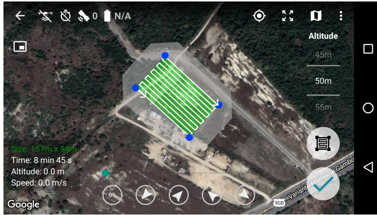
Fig. 3: Screenshot of Altizure, the mobile application used to implement the flight strategy for image acquisition.
