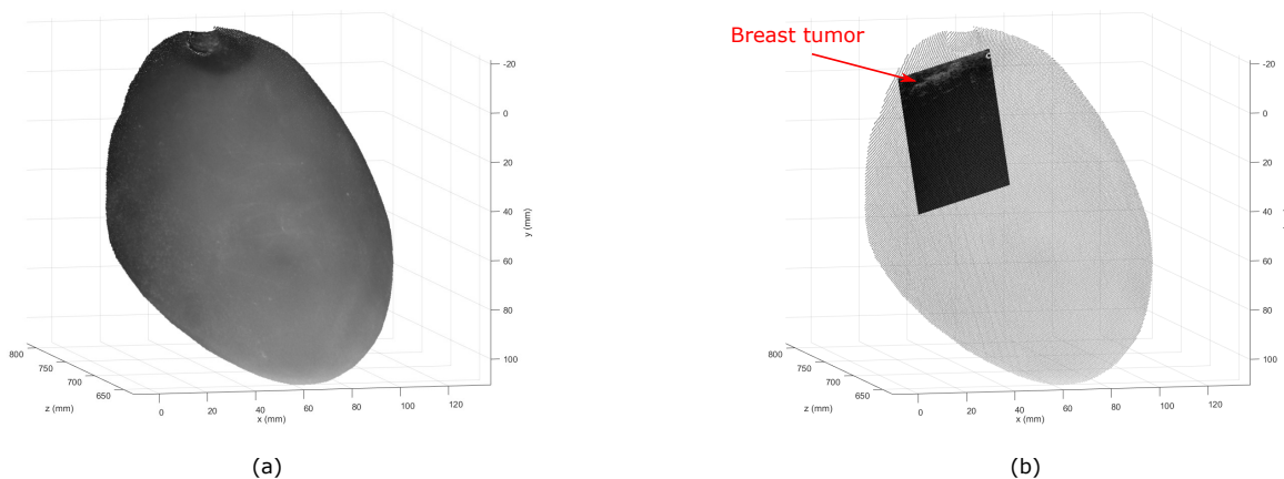
Figure 6. Reconstruction results using FPP and Freehand US: (a) 3D reconstructed surface of the breast phantom. (b) B-scan of a tumor from the breast mapped to the world frame with the 3D phantom surface in the same coordinate system.
